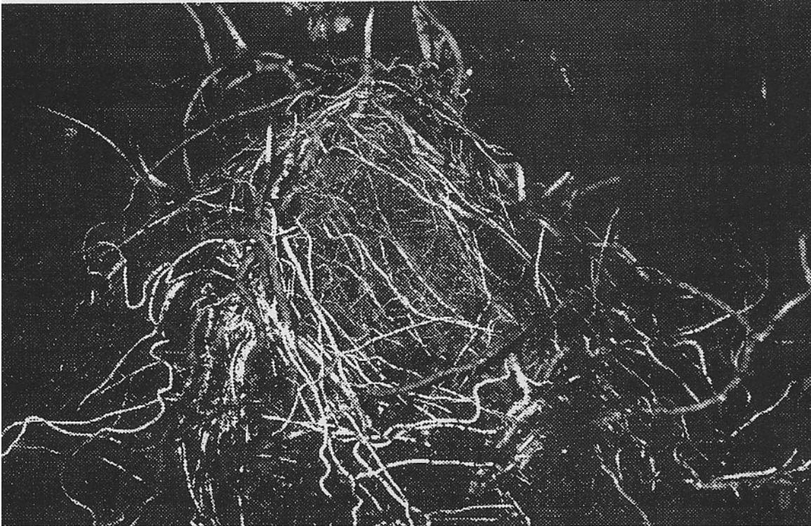
Fig. 4. View of the underside of compost completely infiltrated by roots taken from a test container lined with KEMPEROL® V 210
