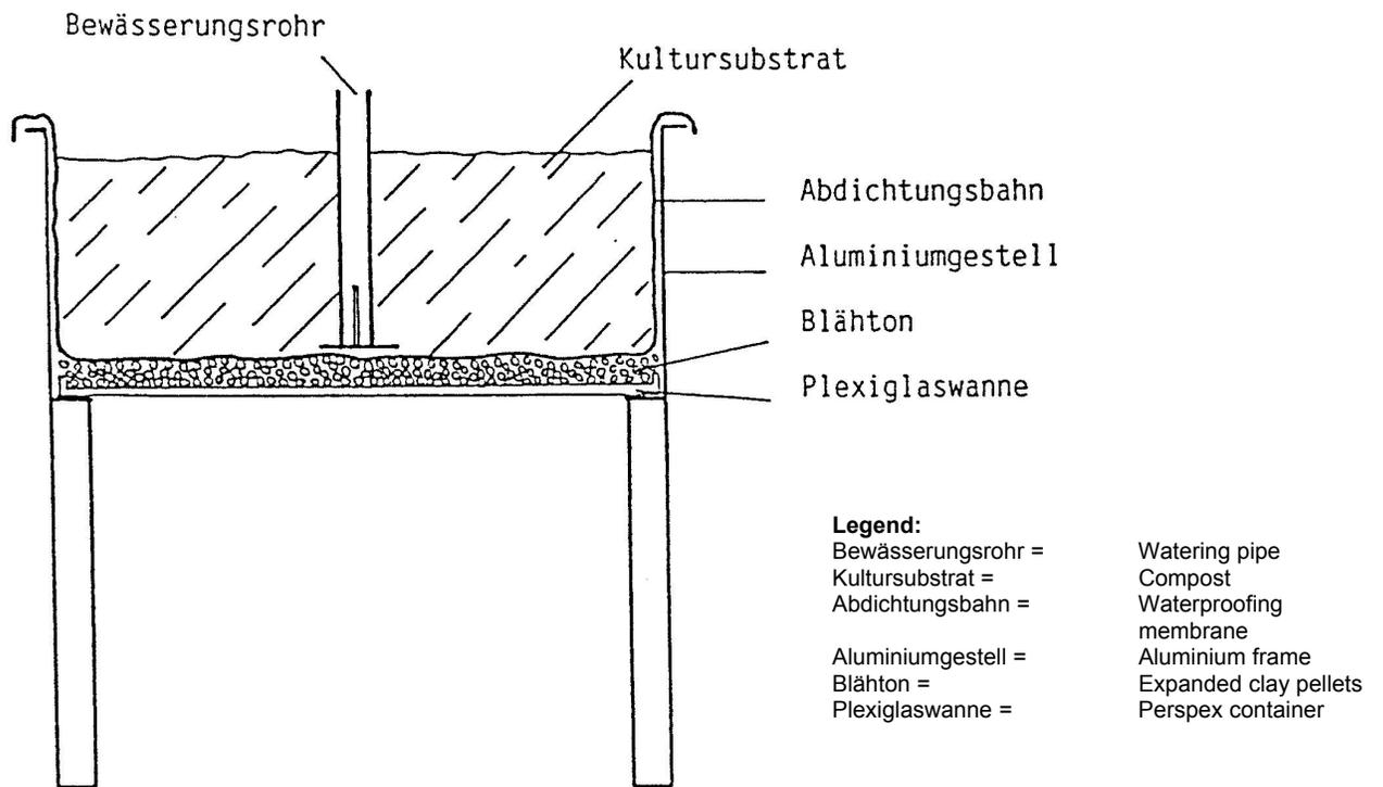
Fig. 1. Section through the test container lined with the test membrane and filled with compost
