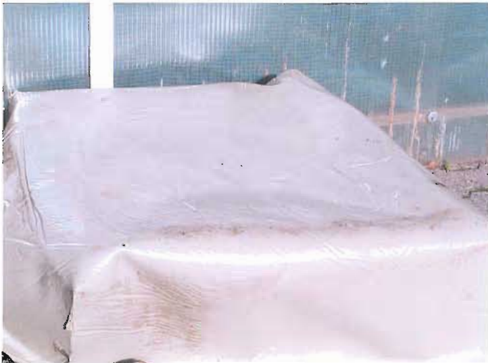
Image 2: Bottom side without root ingress
