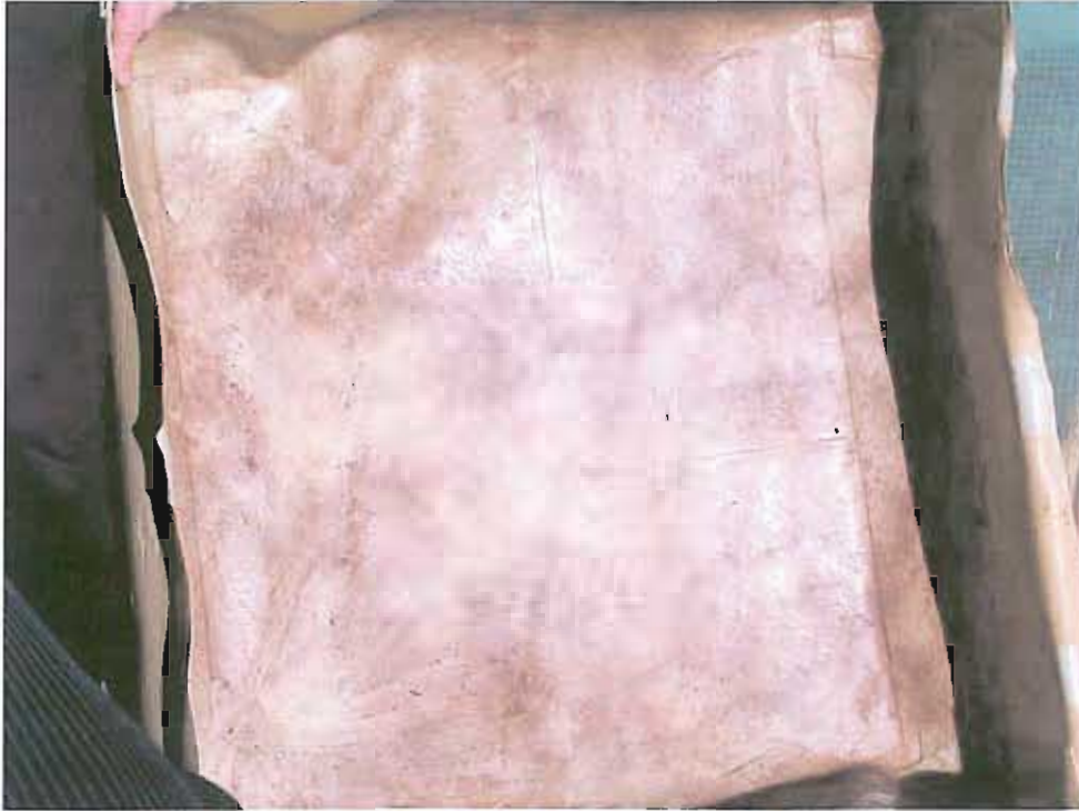
Image 1: Top of membrane without root ingress
