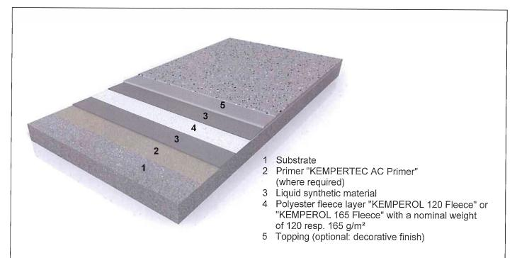
Applicable to the roof waterproofing "KEMPEROL AC Speed" / "KEMPEROL AC Speed+"
