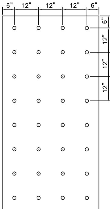
FM-APPROVED MECHANICAL FASTENERS AND PLATES – MUST BE APPROVED BY KEMPER TECHNICAL SERVICES
