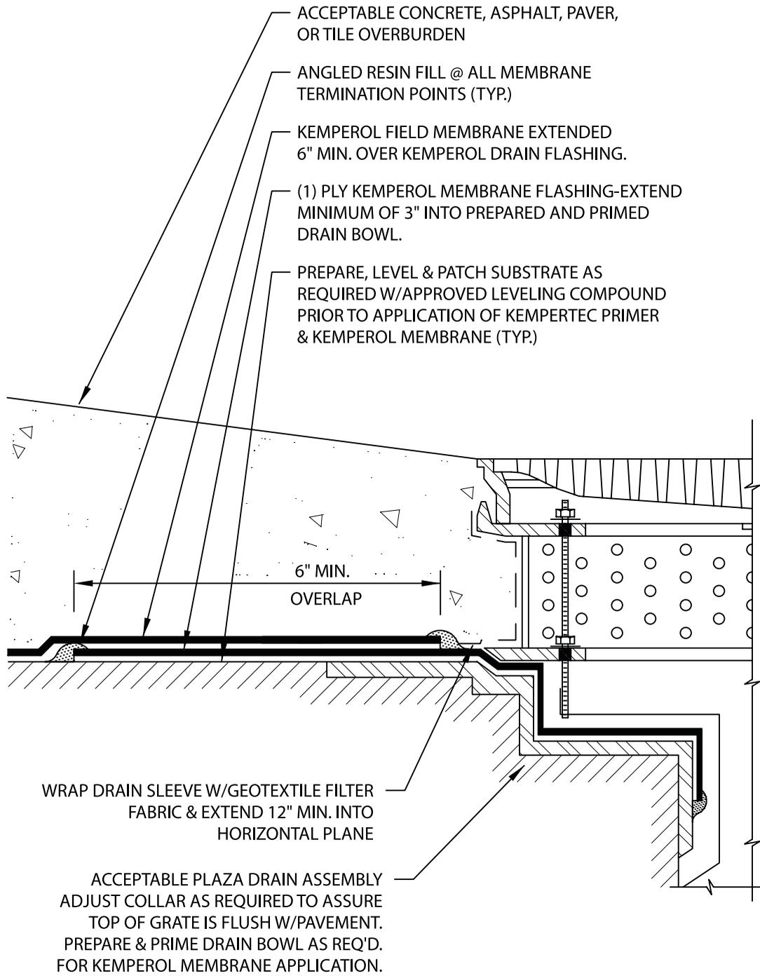
WRAP DRAIN SLEEVE W/GEOTEXTILE FILTER FABRIC & EXTEND 12" MIN. INTO HORIZONTAL PLANE
