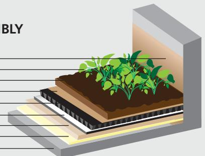
KEMPEROL® 2K-PUR is resistant to UV exposure, is root and rot resistant, and resists degradation by most oils, grease, and other common chemical substances. In addition, KEMPEROL® 2K-PUR is unaffected by standing water and ice, and can be left submerged indefinitely.
