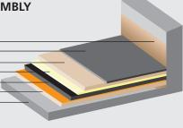
Unlike many other roofing systems, the Kemperol 2K-PUR system incorporates flashings that are made of the same materials as the roofing membrane itself, essentially creating a seamless, self-terminating monolithic membrane that readily adapts to the contours of the substrate.
